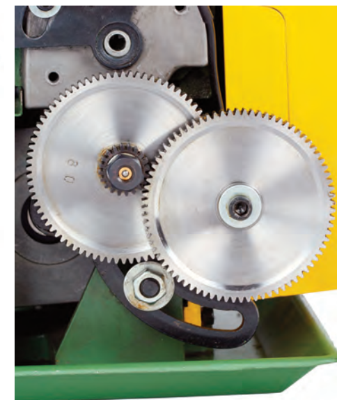
Headstock and thread cutting gears are all steel.
